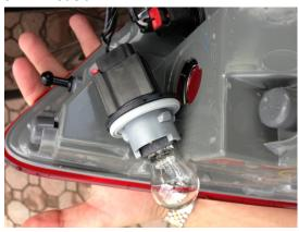
2. Disconnect the taillight plug from the bulb socket and match up the two plugs with the plugs provided on your rear fog conversion kit. Each plug will connect to the rear fog kit connectors without difficulty.
