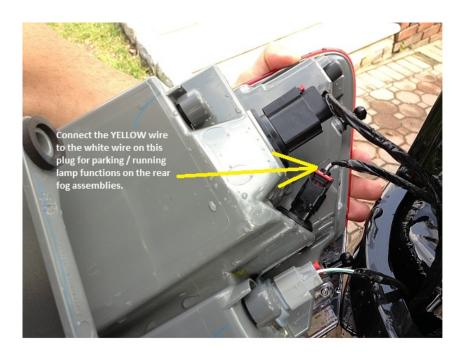
4. Refer to the original WK2 rear fog lamp install manual to complete the remainder of the installation.
