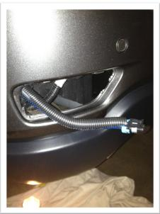
**Step #5** – Connect the matching connectors from the rear fog harness to the stock taillight 3-pin plug and taillight socket. After making the connections and verifying they are secure, tuck / conceal as much of the harness and connections into the body cavity so the taillight will not be obstructed when being re-installed. For proper installation, only two the two plugs for the taillight and reverse should be exposed prior to reinstalling the taillight.
