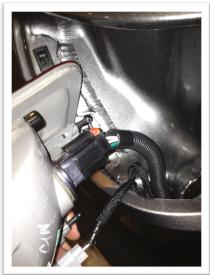
**Step #6** – Connect the appropriate (driver or passenger side) rear fog lamp housing to the conversion harness plug that was routed from the taillight cavity. After making a secure connection to the lamp assembly, install it into the bumper in a reverse fashion of how the reflector was removed. Repeat for the opposite side
