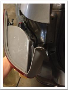
**Step #3** – Starting with the side where the taillight was removed. Reach underneath and behind the bumper and locate the opening in the bumper where the reflector is located. Now locate the outside tab that is closest to the corner of the bumper and carefully push it inwards toward the center of the vehicle. While pressing the tab apply pressure to the inside of the reflector until it that side comes free from the bumper. Remove the reflector from the bumper and place it to the side.
